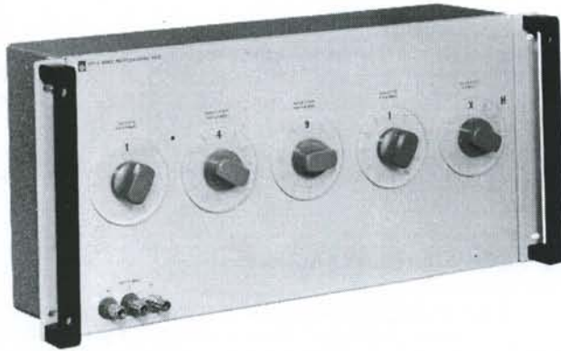
Figure 1-1. Type 1491-G Decade Inductor.
